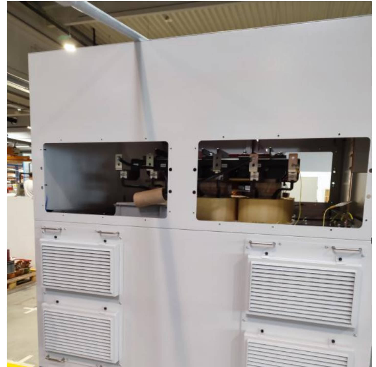
Transformers and inductors in solid state UPS for data centers 15mEuro so far.
